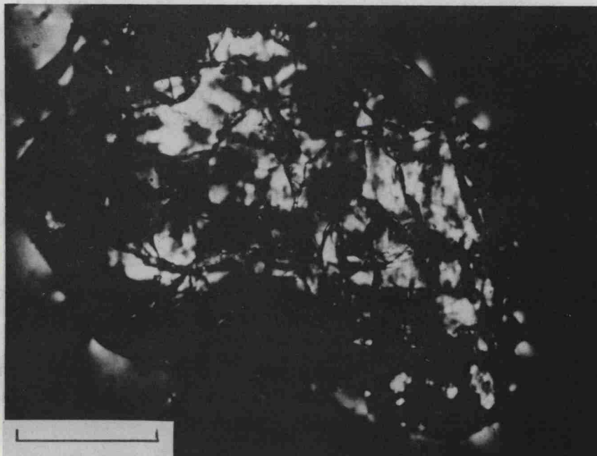
Figure 22B. Same view as Figure 22A; crossed polarizers. The fragment is largely isotropic with some internal birefringence. The birefringence pattern is patchy and irregular rather than spherulitic, suggesting that the birefringence may arise from relict crystalline structure in the maskelynite rather than from post-shock devitrification.
